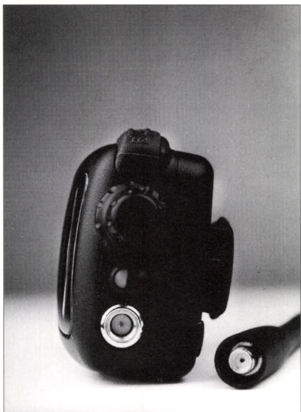
Close up view of the SMA type antenna base socket, and the base of the antenna itself on the Yaesu FT-10R (see text for comments).
